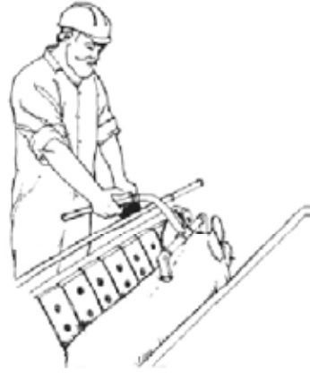
Electric head-to-back cardiac arrest stunner placed in the correct position on a pig in V restrainer.
